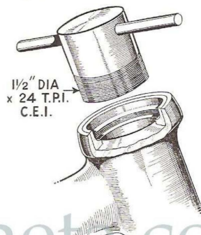
Fig. M44. Steering head ballrace extractor 61-1919.
