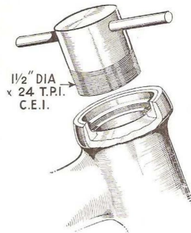
Fig. M44. Steering head ballrace extractor 61-1919.
