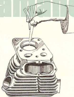
Fig. C.13. Checking piston ring gaps.
