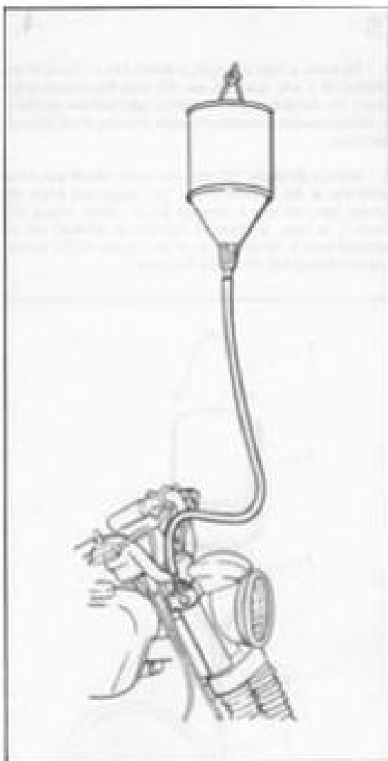
Figure 2-25. Filling Hydraulic Fork with Oil
