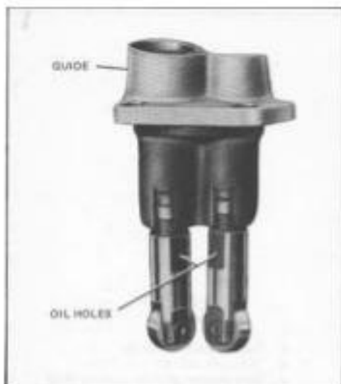
Figure 3-23. Inserting Tappets in Guide
