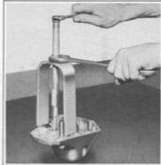
Figure 3-26. Removing Pinion Shaft Cover Bushing
