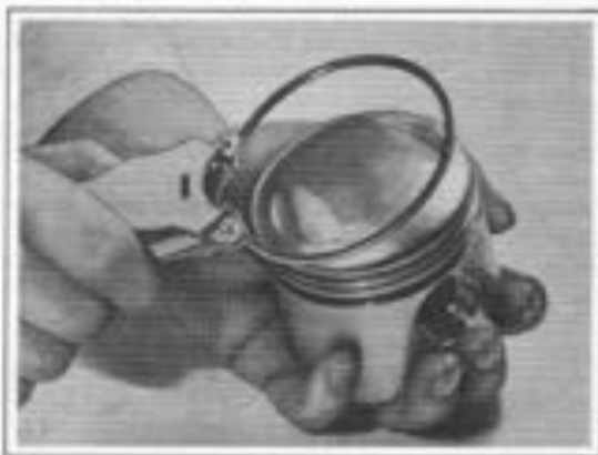
Figure 3-13. Assembling Rings with Ring Expander
