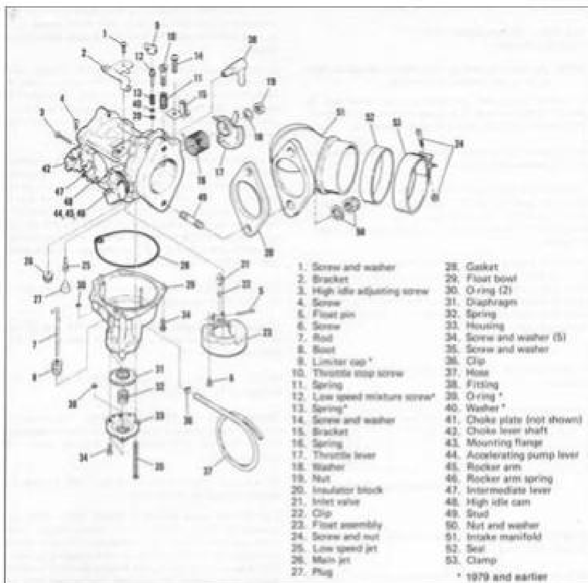
Figure 3-53. Carburetor – Exploded View
