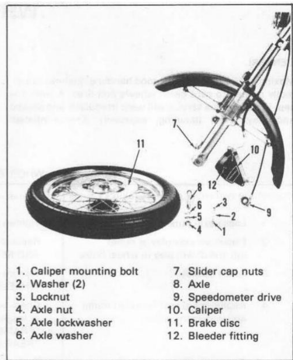
Figure 2-7. Front Wheel Removal (1974 to 1977)
