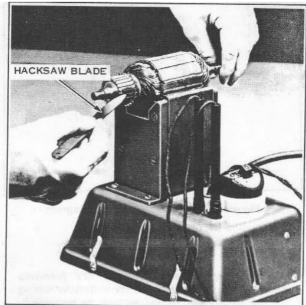
Figure 5-16. Testing Armature for Open Circuit
