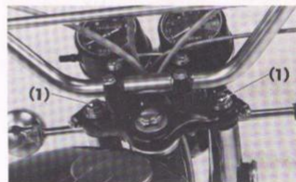
Fig. 2-38 (1) Oil filler plug
