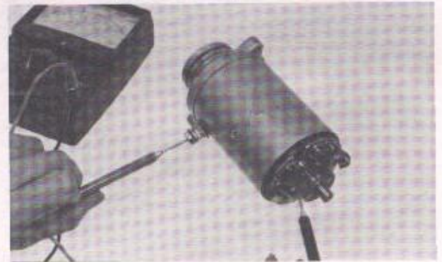
Fig. 5-24 Checking stator coil
