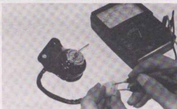
Fig. 5-29 Checking main switch for continuity
