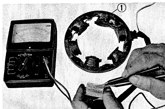
Fig. 152 Stator coil test ① Stator coil
