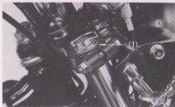
Fig. 5-62 Front forks should be identical in height
