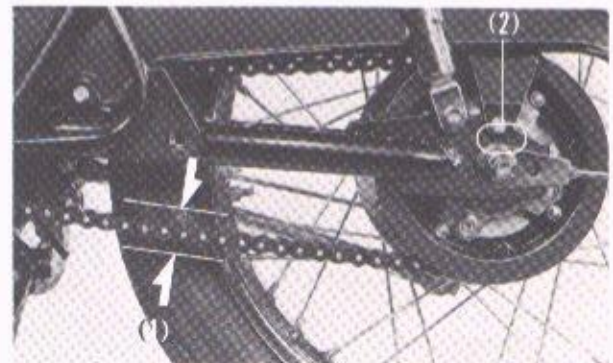
Fig. 4-7 (1) Chain slack (2) Index and reference marks
