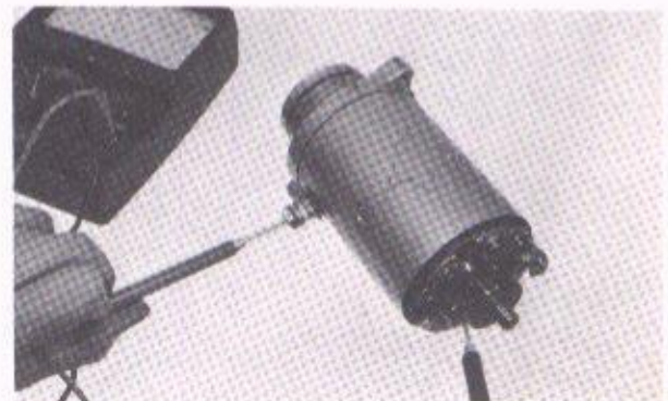
Fig. 6-23 Checking stator coil
