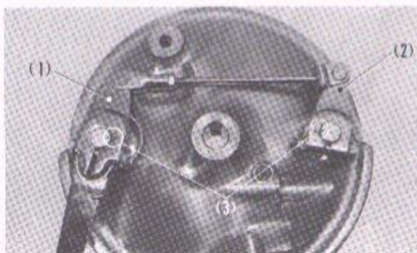
Fig. 5-18 (1) Front brake arm A (2) Front brake arm B (3) Marks
