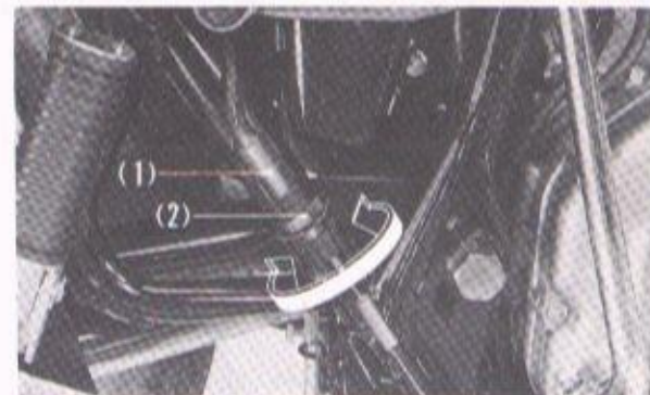
Fig. 6-29 (1) Rear stop switch (2) Adjusting nut
