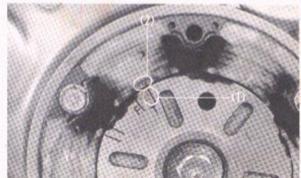
Fig. 3-3 (1) "T" mark (2) Index mark on stator
