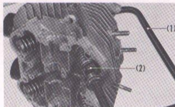
Fig. 4-22 (1) Valve spring compressor (2) Valve cotters
