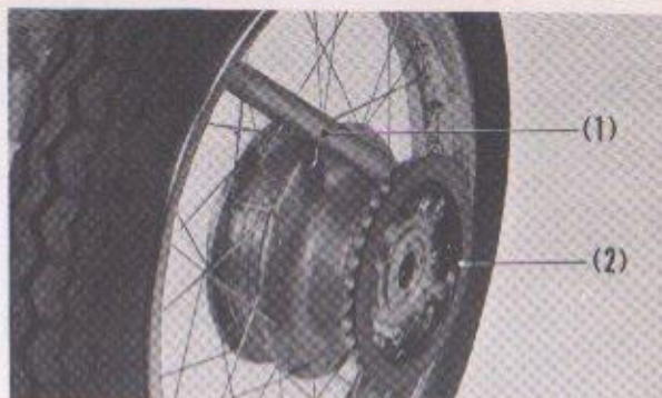
Fig. 5-38 (1) Wood block (2) Final driven sprocket
