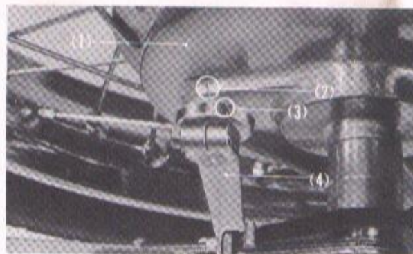
Fig. 3-37 (1) Rear brake panel (2) Reference mark (3) Arrow mark (4) Rear brake arm
