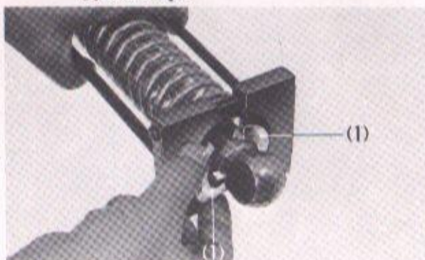
Fig. 5-80 (1) Spring seat stops (2) Rear shock absorber compressor
