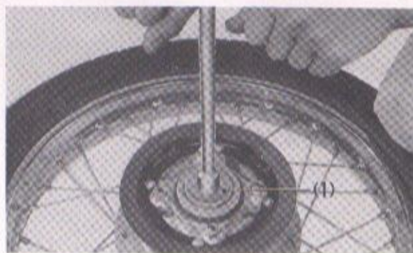
Fig. 5-39 (1) Bearing retainer wrench
