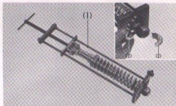
Fig. 5-76 (1) Rear shock absorber compressor (2) Spring seat stoppers
