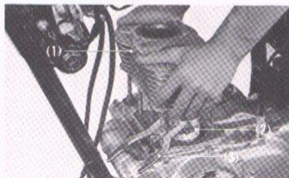
Fig. 4-31 (1) Cylinder (2) Piston (3) Piston ring compressor
