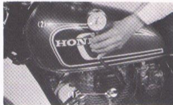
Fig. 3-45 (1) Compression gauge attachment (2) Compression gauge
