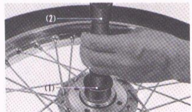
Fig. 5-7 (1) Bearing driver attachment (2) Driver handle
