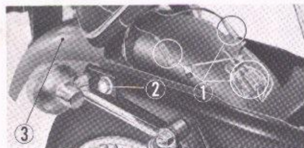
Fig. 5-64. Removing the rear fork
