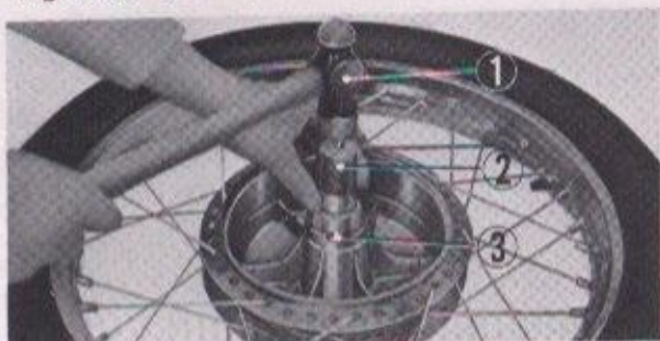
① Hammer ② Bearing driver ③ 6302R ball bearing Fig. 5-90. Driving the bearing
