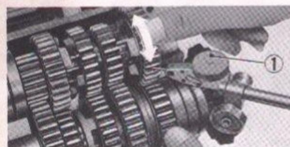
Fig. 4-109. Measuring the gear backlash.
