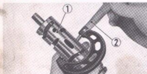
① Gear shift drum ② Micrometer Fig. 4-117. Measuring the outer diameter
