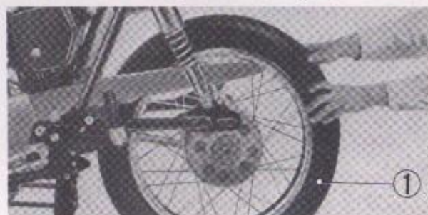
① Rear wheel Fig. 5-127. Removing the rear wheel from the frame
