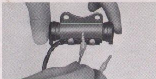
Fig. 6-20. Short-circuiting of the condenser
