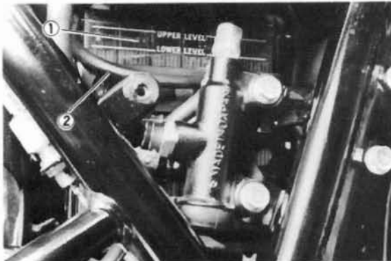
1. Battery 2. Battery vent hose
