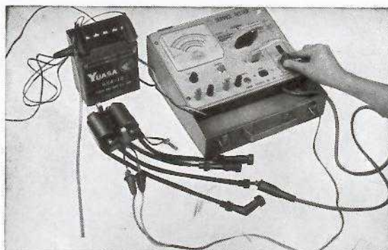
Fig. 7-8 Ignition coil test
