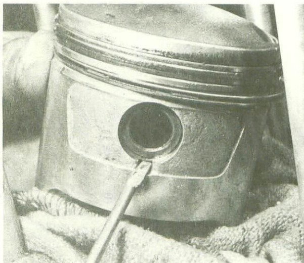
8.1 Prise in groove to release circlip
