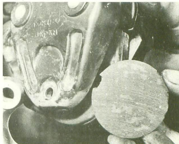
15.2 Pad 'A' being removed
