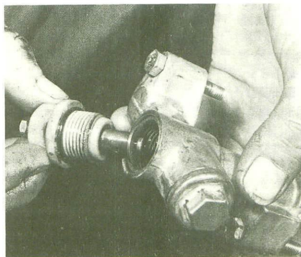
17.1A Removing pressure switch from body
