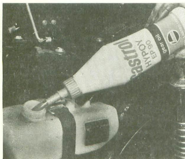
RM11 Topping up chain oil tank
