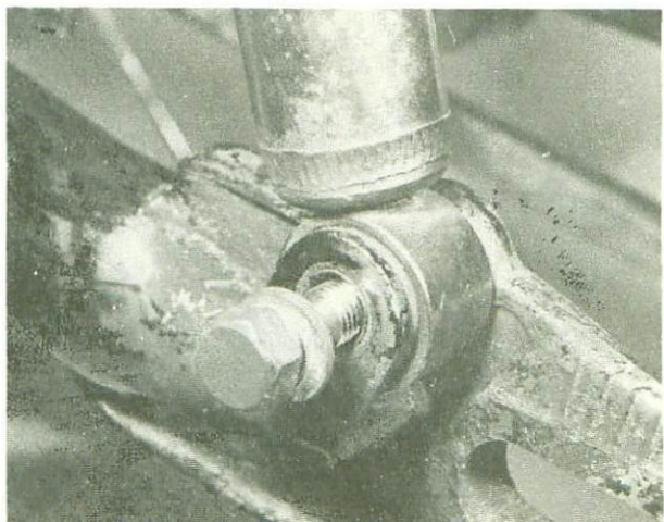
9.4 Remove bottom suspension unit bolts
