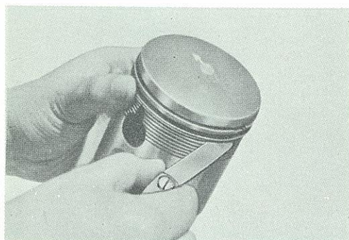
Fig. 8-11-4 Checking side clearance
