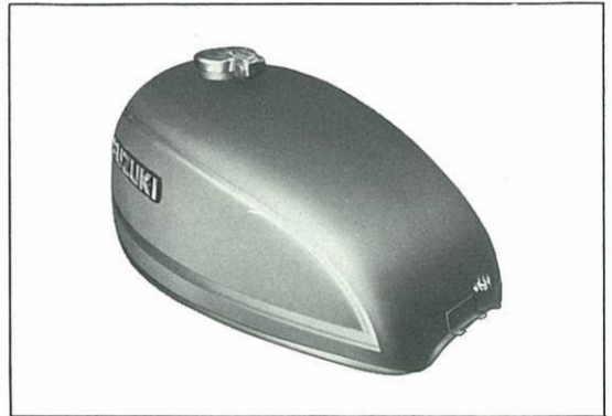
Fig. 12. T500 Fuel Tank 14 lit. (3.7/3.1 US/Imp gal)
