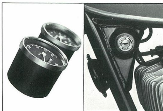
Fig. 10. Meters and Ignition Switch in T500
