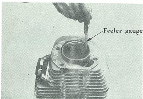
Fig. 8-11-3 Measuring end gap
