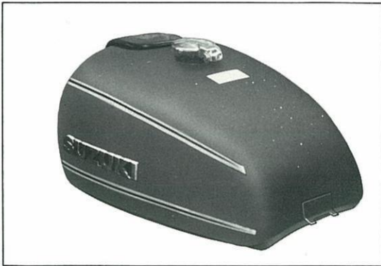
Fig. 11. GT500 Fuel Tank 17 lit. (4.5/3.7 US/Imp gal)
