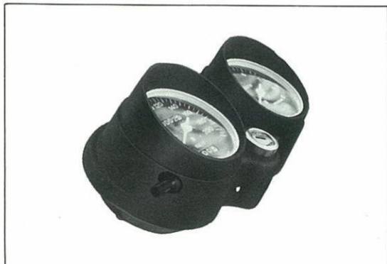
Fig. 9. Meters and Ignition Switch in GT500
