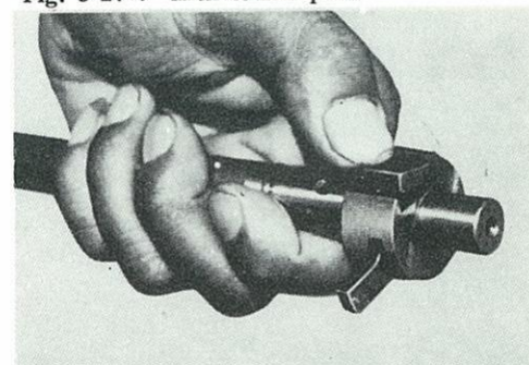
Fig. 8-24-5 Check kick starter pawl roller operation
