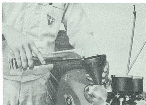
Fig. 9-6-9 Pouring fork oil
