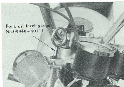
Fig. 9-6-10 Measuring fork oil level
