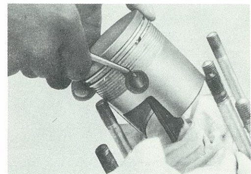
Fig. 8-8-1 Removing piston pin circlip
